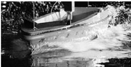
54% lower significant vertical accelerations in bow area at 25 knots compared to conventional hulls. Even more at 30 knots.
