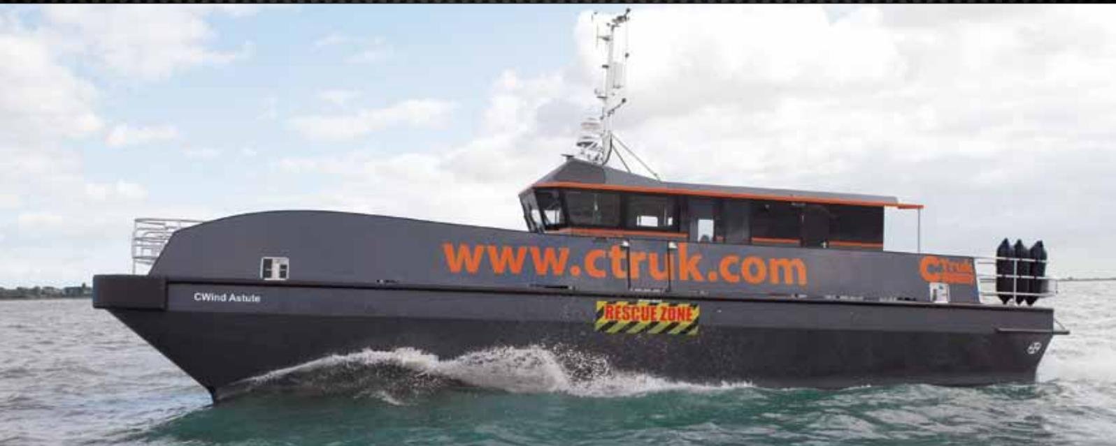
CWhisper was designed to dramatically improve the comfort of technicians transiting out to offshore wind farms. Motions are approximately a quarter of those of conventional catamarans, significantly increasing the current wave height limits for technician transfer and thereby reducing downtime due to adverse weather. CWhisper is also extremely cost-effective, with a measured fuel consumption of less than 100 litres per hour at 20 knots.
