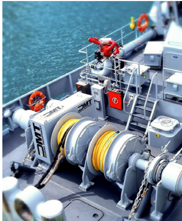
Electric Towing Winch delivered to equip a 60T Mtug
