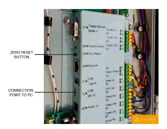
To zero the system you need to press and hold the button for 5 seconds and this will remove any offset on the shaft. The torque display will now read 0 kNm.
