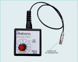
Please note that it is only possible to use the strain gauge simulator whilst the shaft is static as you will need to connect to the on shaft transmitter.
