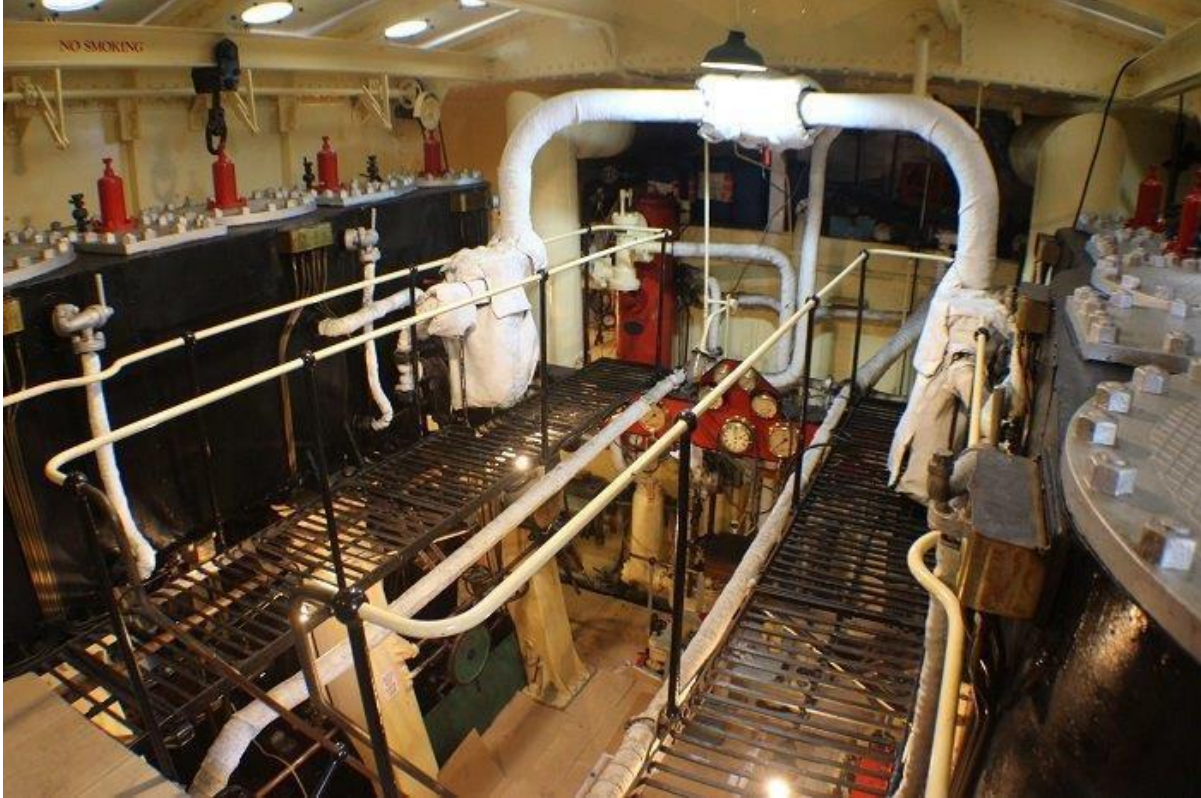
In the engine room: A seawater-circulating pump, fire and bilge pump, backup general-service pump, power generator, two main winches and steering cap-off are all powered by the hush of steam.
