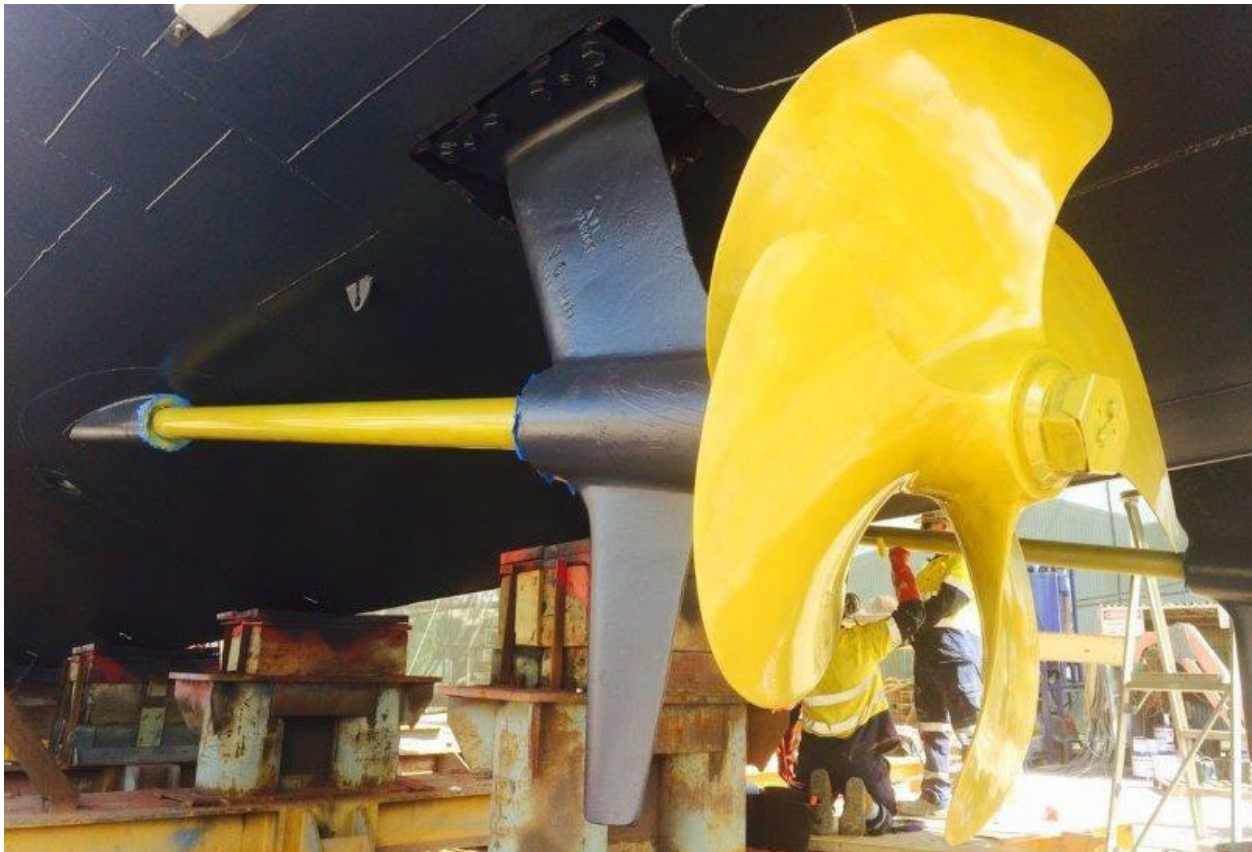
Te Matilli's propeller and shaft are now protected by the gold-standard foul-release coating.
