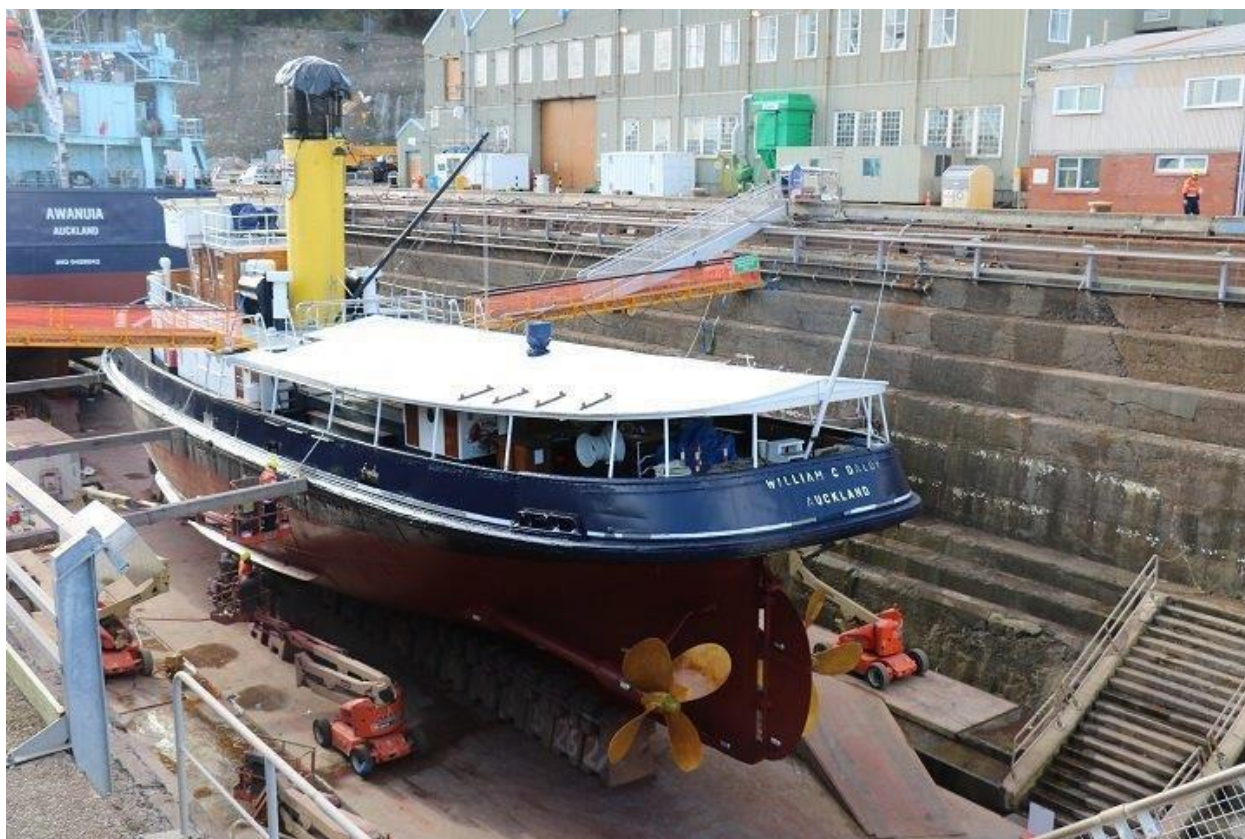
William C Daldy steam tug's propellers protected by Propspeed foul release coating
