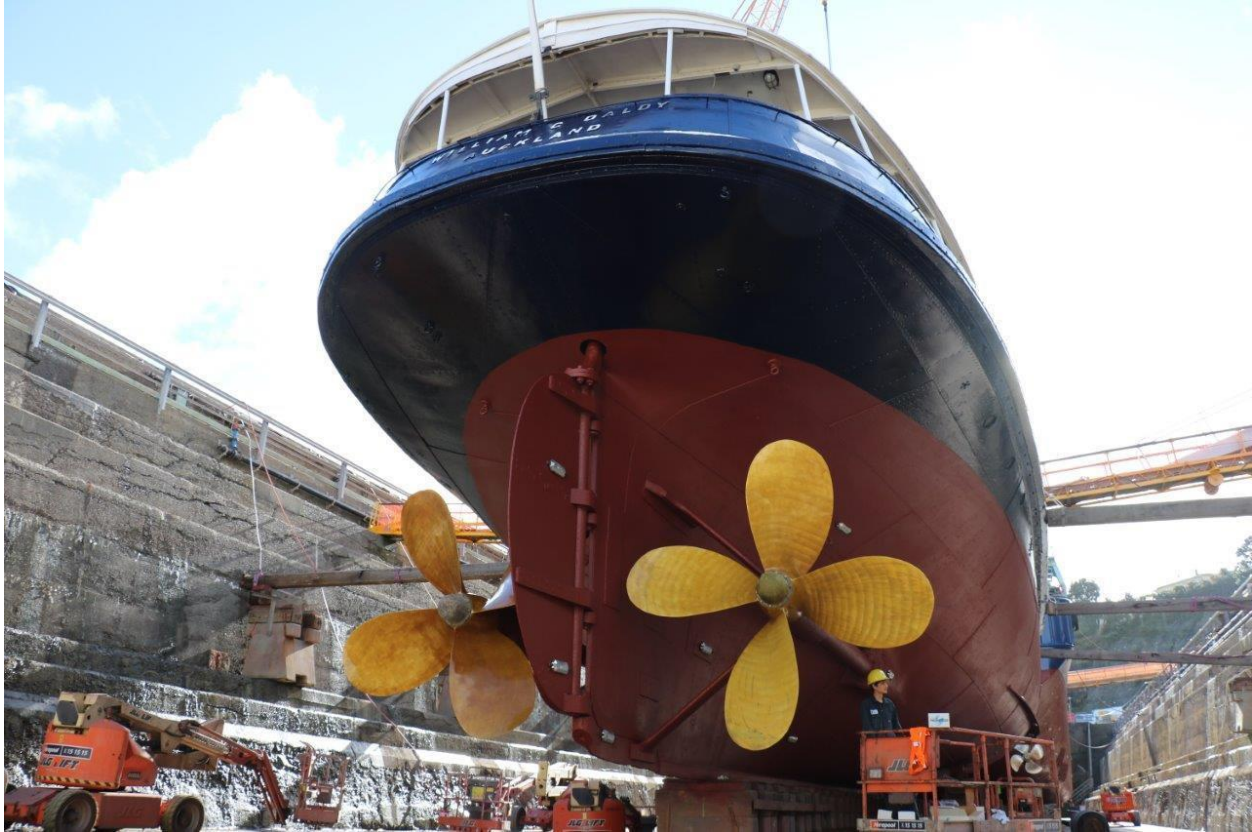
A beautiful behemoth: Each 3.4-ton propeller is nearly 12 feet (3.58 meters) in diameter, generating 980 ihp at 115 rpm.
