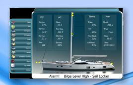
system will simply use its existing dual redundant Ethernet cables to send the control signals. Systems are designed and configured to your wishes, then given factory acceptance test sign off by the relevant classification society (e.g. Lloyds) before being fitted to your vessel. Lockouts can be programmed into the system to stop undesired operations being carried out depending on pre-set criteria.
