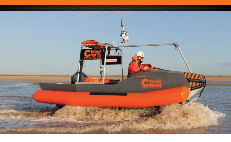
CTruk Avenger is an amphibious rescue and survey vehicle that can be carried on and launched from a CTruk 20T MPC or other mother ship.
