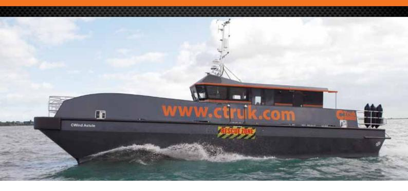
CWhisper was designed to dramatically improve the comfort of technicians transiting out to offshore wind farms. Motions are approximately a quarter of those of conventional catamarans, significantly increasing the current wave height limits for technician transfer and thereby reducing downtime due to adverse weather. CWhisper is also extremely cost-effective, with a measured fuel consumption of less than 100 litres per hour at 20 knots.
