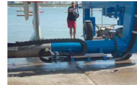
Variable width frame for accurate boat lifting and parking. This feature also acts as a pivot bearing when traveling over uneven ground
