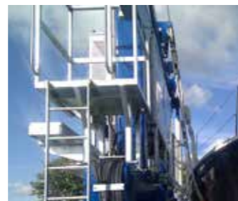
Raised drivers stand and access walkway constructed from 316 stainless and galvanised steel
